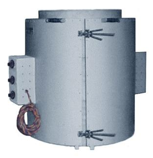
Drum Heaters are mobile ovens heated by flexible surface heaters. They are made in rugged designs and stand normal usage in chemical industries. They can be used for heating the contents of drums kept in the vertical or horizontal positions.
